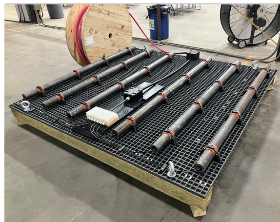
TIMBERSLED™ IS AN ULTRA-LOW PROFILE ICCP SLED Perfect for very shallow water applications, it's only 300 millimeters tall.
