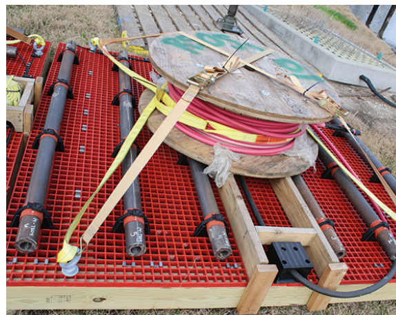
ANODES DESIGNED FOR SHALLOW FRESH OR BRACKISH WATER Suitable for any seabed type.
