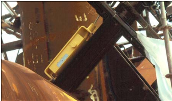
DR-2 mark 1 in situ; the casing has been replaced by black Delrin on the current version
