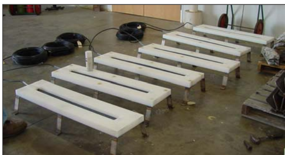
Floor-mount anodes for a potable water tank
