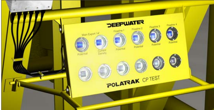
The SunStation monitor, here shown on a deep water monitoring panel (solar panels below in separate housings)
