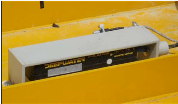
The DR-2 is equipped with one Ag/AgCl and one Zn reference, for unparalleled accuracy.
