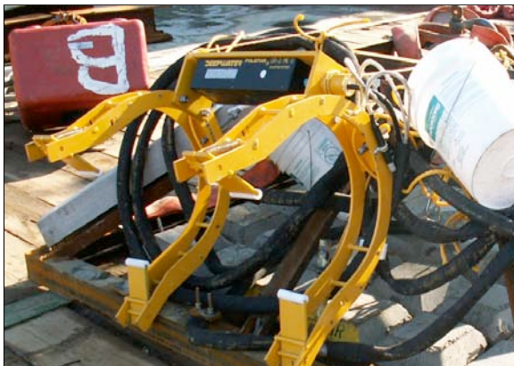
DR-2 to be retrofitted to a subsea pipeline, attached to two RetroClamps
