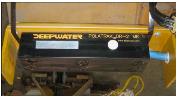
DR-2 in production; the casing is black Delrin on a carbon steel mount.
