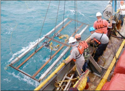
RetroSled w/ 2 clamps being overboarded
