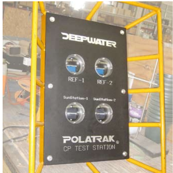
The new SunStations house the readout and solar panels separately.
